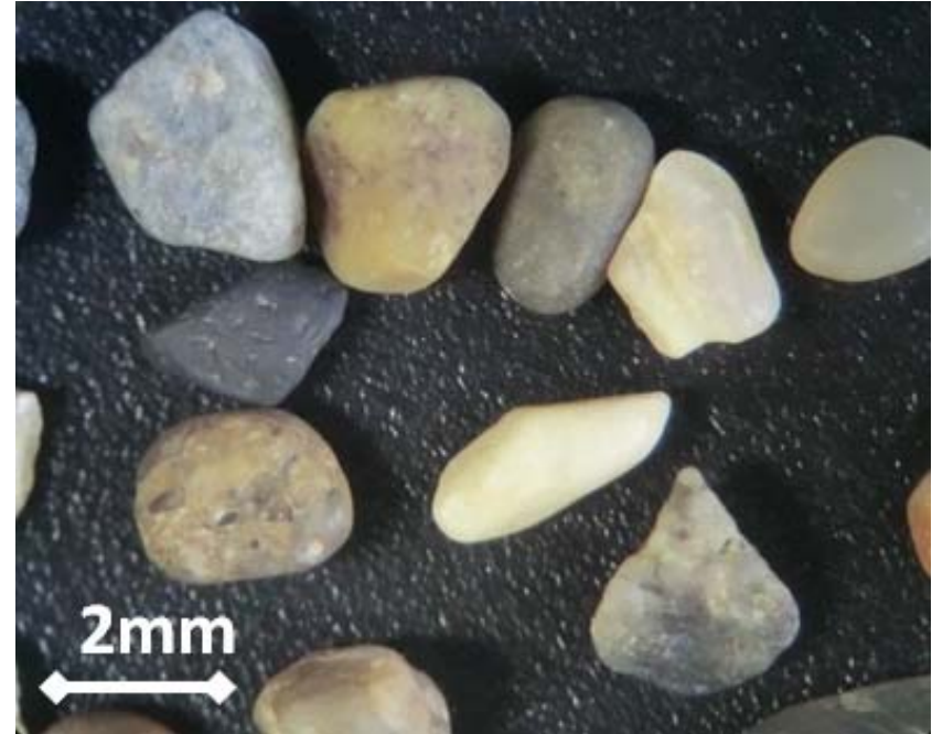
Kashima sand river sand 96.3% \text{SiO}_2 D_{mean} = 2.08\text{mm} round
