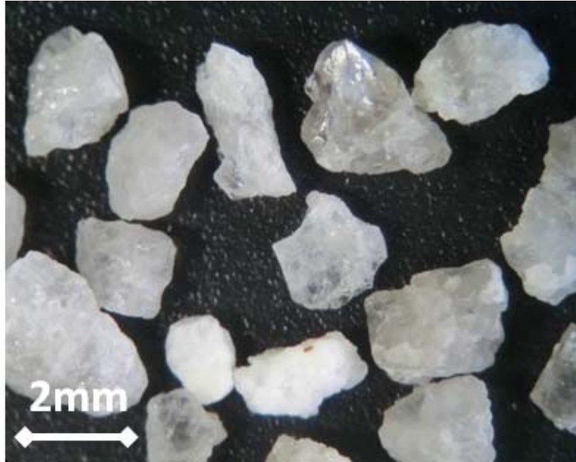
Gifu sand mountain sand 90.2% \text{SiO}_2 D_{mean} = 2.38\text{mm} angular
