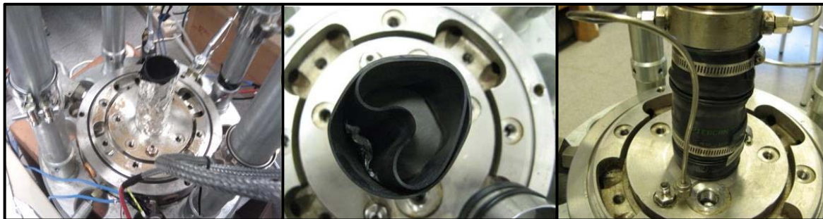
Triaxial/isotropic cell (25 mm in height, 50 mm in diameter)
